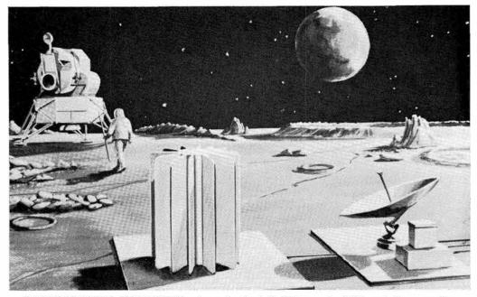
SNAP-27 ISOTOPIC GENERATOR is shown in the left foreground of this artist's conception of how it will be placed on the surface of the moon to provide power for the Apollo Lunar Surface Experiment Package. SNAP-27 is under Sandia's technical direction.
